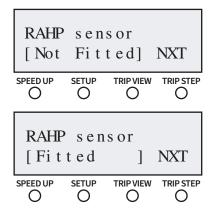
Press the **SETUP**> button again. The "RAHP sensor" window is displayed providing control of Outdoor Fan speed. Press **TRIPSTEP**> to toggle between "Not Fitted" and "Fitted". "Not Fitted" means the Outdoor fan runs at one speed only. "Fitted" means with RAHP inputs, the Outdoor fan can operate with LOW or HIGH speed based on the measured Outdoor coil pressure during Cooling mode only. RAHP will be ignored during Heating hence the outdoor fan will be forced to run in HIGH speed.
