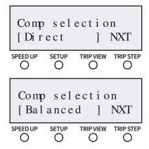
Press the **<SETUP>** button again for "Comp selection" screen. This allows the user to choose a simple load balancing behaviour, called lead/lag, if desired.
