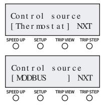
Pressing the **SETUP**> button again gives a choice of "Control source". Possible choices are either "thermostat" or "MODBUS" control. Pressing the **STRIPSTEP**> button toggles between "Thermostat" or "MODBUS" control. (Choosing Thermostat control does not remove the ability
