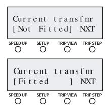
Press **SETUP**> button again to give access to "Current transfmr". This enables the user to set the presence of a Current transformer (CT). The use of a CT is purely for information. It does not control anything in the system. Press **STRIPSTEP**> to toggle between "Not Fitted" and "Fitted". "Not Fitted" means the Current Transformer is not used. "Fitted" means the Current Transformer is used and connected to the LT1 controller for measuring the current consumption of compressor(s).
