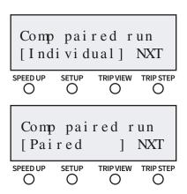
Press the **SETUP**> button again for "Comp paired run" window. This allows the compressors to be run as a pair only with a 10 second interval between lead and lag compressor start, or as individual only. If "paired" is chosen, connect thermostat to st 1 connection on control board. Press **TRIPSTEP**> to toggle between "Individual" and "Paired".
