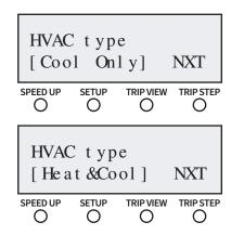
Press the **SETUP**> button again. "HVAC type" is displayed allowing the user to choose between a "Cool Only" or "Heat pump" (Reverse cycle) system.
